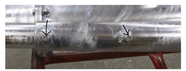
Release the four screws that secure the cover tube to the pump housing.
