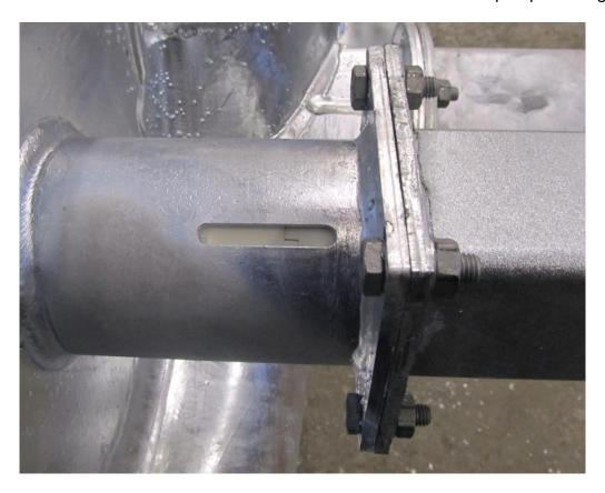
Pull the cover tube away from the pump housing that the storage comes to the view.
