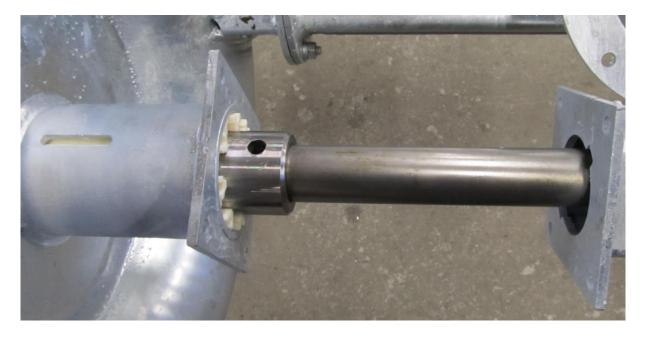
Use a screwdriver or something similar and push out the four plastic bearings. Remove them from the shaft.
